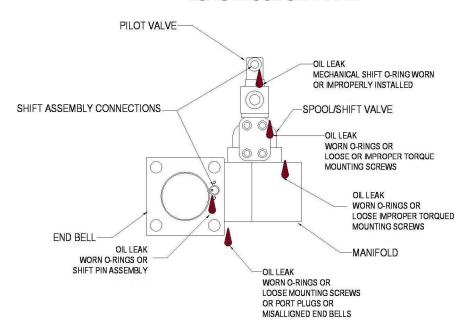
NOTE: Loose fittings can be the cause of any leaking connections. Long and short block intensifiers are broke in to minimize the probability of this happening
