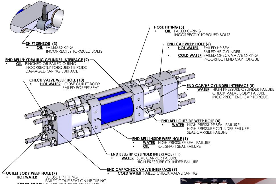
FAILED CONE SEAT ON HP TUBING
