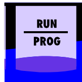
Function key: In automatic work mode, allows you to enter programming and return to execution In programming work mode, allows you to switch between the program cuts and select program displays
