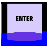
Function Key: Calling up program No. Scrolling the cursor Storing data Storing programs Selecting programs Storing parameters
