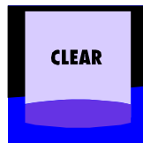
Function Key: In automatic work mode, allows you to delete the last program carried out by loading the new one to be carried out In programming work mode, allows you to delete existing or incorrect data When entering cutting or machine parameters, allows you to delete existing or incorrect data
