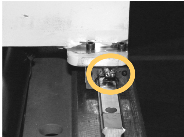
Linear bearing grease nipples. Four in total, two at the front of the carriage and two at the back of the carriage, hidden by the carriage cover.
