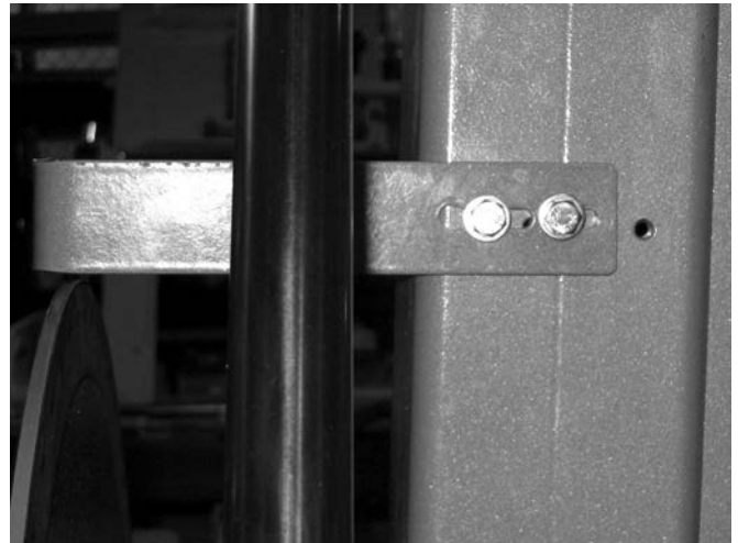
Scale pointer bracket shown at the 90° head position.
