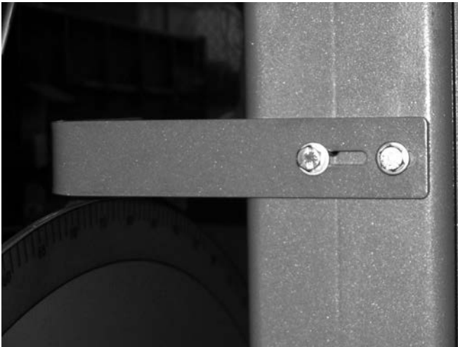
Scale pointer bracket shown at the 3° canted head position.
