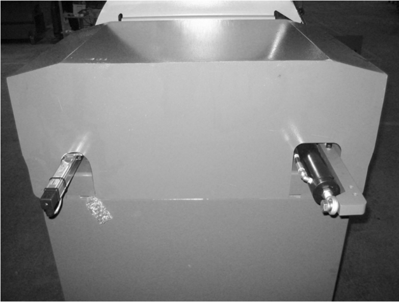
View of the head potentiometer and cylinder after re-installation.
