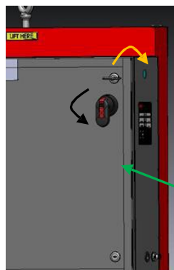
Figure 2.4 Open the door of the Main Electrical Control Cabinet.
