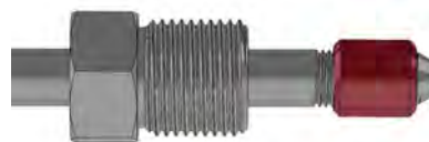
Incorrectly installed collar: The collar interferes with the seal surface.
