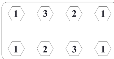
Figure 3 Nut-Loosening Sequence for Removing Clamp Plate from High-Pressure Assembly
