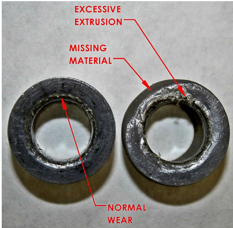
Figure 13 Dynamic Seal Inspection
