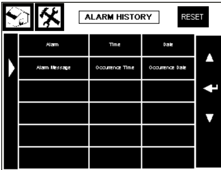
Figure 4-10: Alarm History Screen
