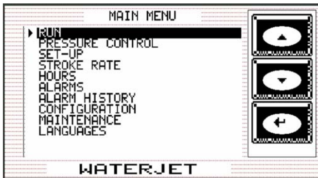
Figure 1-3: Control Panel Main Menu
