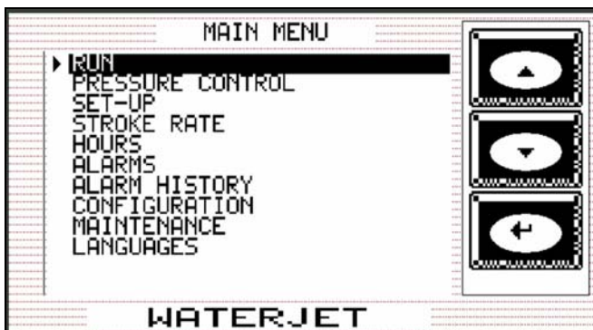
Figure 1-3: Control Panel Main Menu
