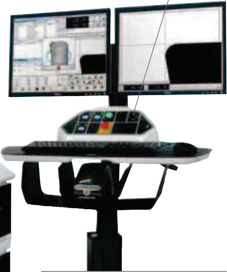
Industrial grade controls for the spindle disk brake system, the 4-position index, the mechanical tool clamping and all other controls are conveniently positioned on the new cockpit system.
