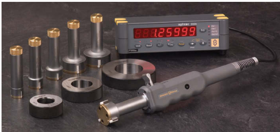
Ultima Gaging System shown with Sylvac digital display. See the display section on page 000 for information.
