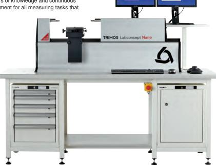
The uncompromising design of the Labconcept Nano offers an ideal and performing platform for checking and calibration of all kinds of gages and measuring instruments. Checking of internal and external dimensions will be done as a fully automatic procedure by the three motorized axis XYZ and the legendary simplicity of use of the Trimos® WinDHI software.
