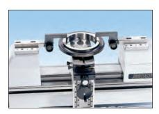
Checking of ring gages from dia. 0.473"(12mm) to 10"(250mm) using table (54-197-011-0), clamps (54-197-142-0) & L-probes (54-197-162-0)
