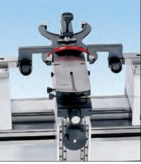
Checking of snap gages with range from 0.473 to 6"/12 to 150mm using table (54-197-011-0), snap gage holder (54-197-014-0) & L-probes (54-197-162-0)
