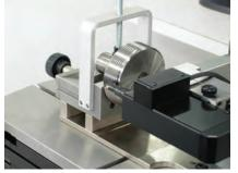
Checking of taper thread plug gages
