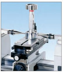
Checking of plug gages and threaded plug gages from dia. 1.18" to 10"/30 to 250mm using table (54-197-011-0), clamps (54-197-142-0), small  $\varnothing$  anvils (54-190-806-0) & thread wires (54-197-007-0)
