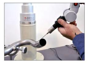
Pipe measurement with touch probe
