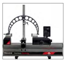
Checking of external micrometer held on a support (TA-SU-309, TA-SU-309, TEL5)
