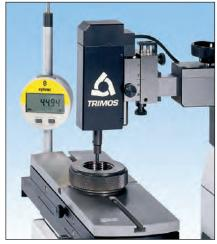
Checking of threaded ring gages from pitch 0.7 to 6mm/48 to 4 threads per inch (max. internal dia. 7.08"/180mm) using table (54-197-011-0), clamps (54-197-142-0), Internal measuring device (54-197-074-0) & T-Ball probes (54-197-075-0)
