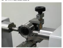
Checking of thread plug gages
