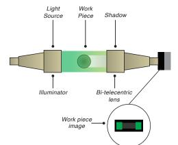
The contour of the workpiece is reproduced in the software and all the various elements shown can be measured statically (without part rotation) or dynamically (with part rotation) when geometrical features such as run-out or concentricity must be measured.
