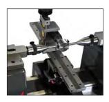
Checking of thread plug gages, max. M100/ø4", length 280 mm/11") (TELb, 3P/ 0.17-3.2/ S6.5, LABC15)
