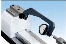
Checking of dial indicators and dial comparators up to 2"/50mm range using dial indicator holder (54-197-015-0)
