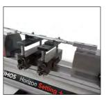
Setting of 2 point internal measuring equipment (TELMA7)
