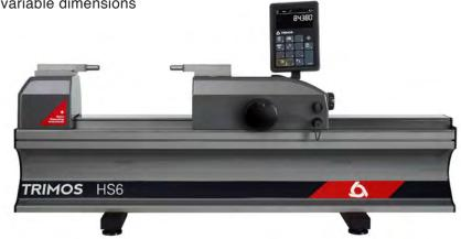
Fowler Trimos proposes a complete range of instruments from 500mm to 3000mm. All measuring ranges are direct, which means that the whole measuring range is available without adjustment or intermediary recalibration. A large selection of easily interchangeable accessories completes the possible applications and guarantees a correct positioning of the instruments to be calibrated.
