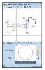
**FT2-E:** Complete TOUCH SCREEN DRO with 2D Fusion Touch software as above. Built-in optical edge detection allows data points to be taken 'on the fly' as the projected image is passed under the screen-mounted fibre optic sensor. An internally mounted edge sensor is available as an option on all 'R' series projectors.
