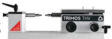
High accuracy is guaranteed by perfect instrument construction and the Heidenhain measuring system. The simplicity of the instrument and its ease of use allows precise and quick performance of all measurements. Adjustable Measuring Force is suitable for measuring thread members utilizing the 3 wire method.
