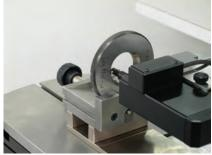
Checking of taper thread ring gages
