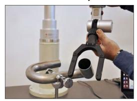
Pipe measurement with laser fork
