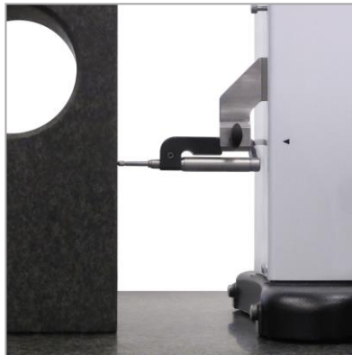
Perpendicularity measurements with electronic probe
