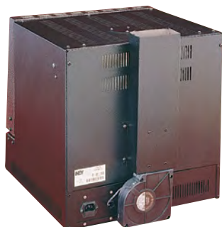
Rear view of exhaust/blower system
