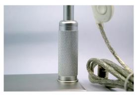
The endoscope can be moved up and down by turning the pillar (see left photo) for getting larger photo area or smaller photo area.
