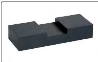
flat anvil for test block (included)
