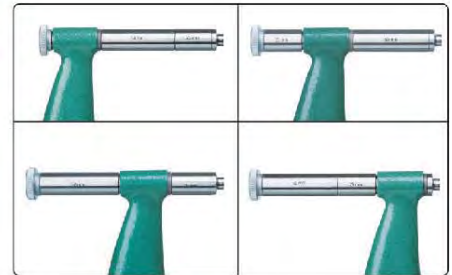
adjust collars for different measuring ranges
