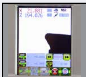
Automatic Edge Targeting makes measuring fast and accurate.
