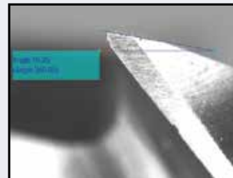
Cylindrical cutter with 4 cutting edges, diameter 6mm. Side view (chest): measure the propeller screw angle and rake angle, important to determinate to suit the type of application and the type of material being processed.
