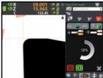
CNC Automatic measurement feature provides the utmost consistency for diameter and length measurements.
