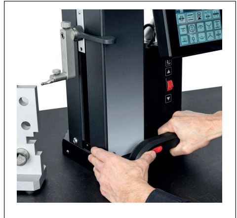
Fig. 8 Moving the height measuring instrument using the activated air bearing
