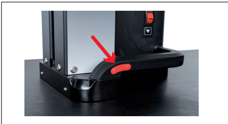
Fig. 6 Button for activating the air bearing
