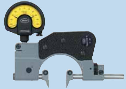
840 FM with jaws for gear tooth span and thickness
