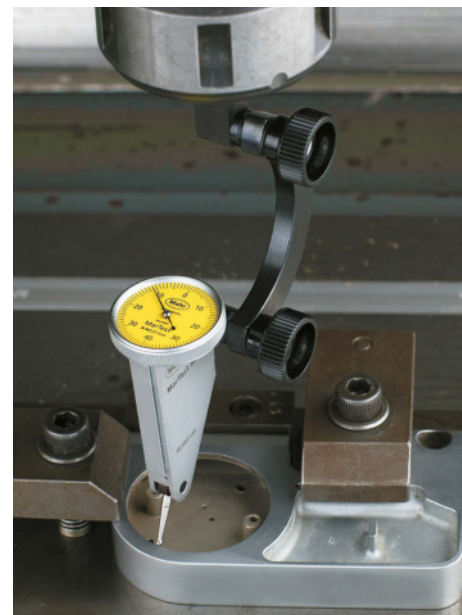
Centering of a bore
