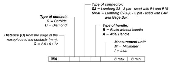
**Example:** Need to order an M4 with C=2.5 mm, carbide contacts, E4N connector, without handle, max. Ø 38.735 mm (1.525 inch), min. Ø 38.710 mm (1.524 inch).
