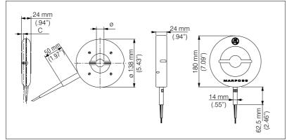
The M4 comes with various C measurement point distance values that allow great flexibility in the measurement position. The C dimension comes in 2,5 mm for close to flange measurements, in 6 mm for normal measurements and in 12 mm for bottom measurements.
