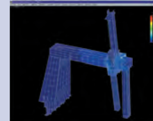
The machine structure has been optimized using FEM (Finite-Element Method) and modal analysis.
