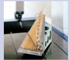
CMM calibration tool using the virtually zero thermal expansion glass gage
