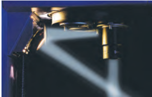
Adjustable / oblique switchable surface illumination
