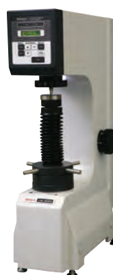
HR-430MS Rockwell/Rockwell Superficial hardness testing machine Motorized Loading Motor drive - Automatic start model
