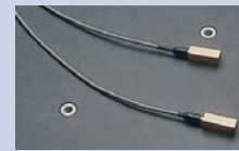
Temperature compensation system (photo: temperature sensors)
