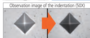
Stray light reduction around the indentation
