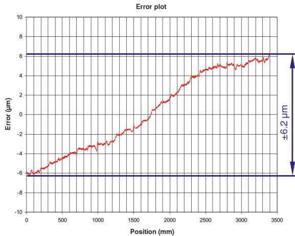
Example accuracy test result of 3400 mm length of RTALC scale
