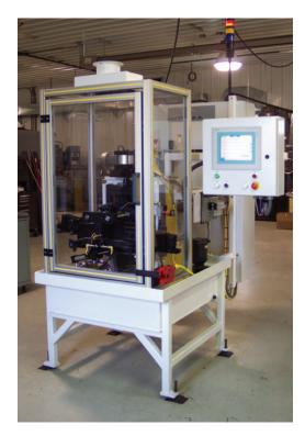
These machines and their unique process remove nicks, burrs, heat treat scale and other foreign matter from the gear tooth flanks.
