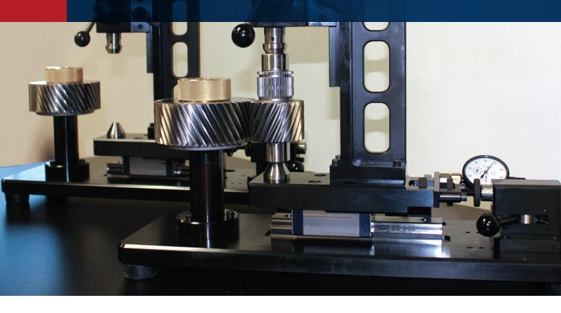
Veit Tool & Gage manual and motorized double flank Gear Roll Test Fixtures, have a proven long quality record in the gear industry. They offer superior accuracy and repeatability, along with a very broad range of applications.
