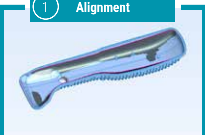
Alignment actual- to nominal component
