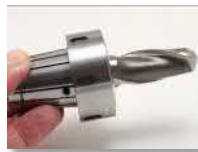
Fully insert cutter into the collet
