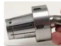
Once the pin is fully inserted pull out on the cutting tool so the back of the flat is tight against the pin Use safety gloves if required
