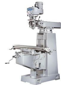
TMV Knee Type Vertical Mill with Box Ways
