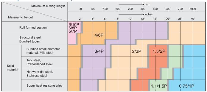
Note 1: When cutting profiles or structurals, it is desirable that at least 2 teeth are in contact with the material being cut at all times. This will prevent chipping and stripping of the teeth and eliminate premature blade failure.
