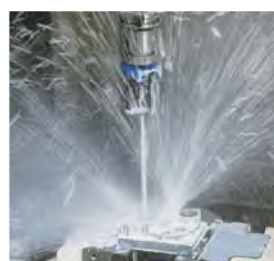
High-pressure washing with center-through coolant
