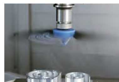
Blows away cutting chips with powerful air pressure
