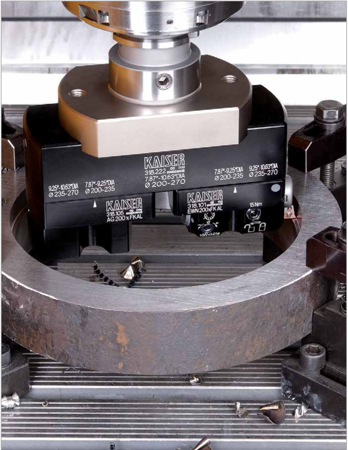
B.4 LARGE DIAMETER BORING
