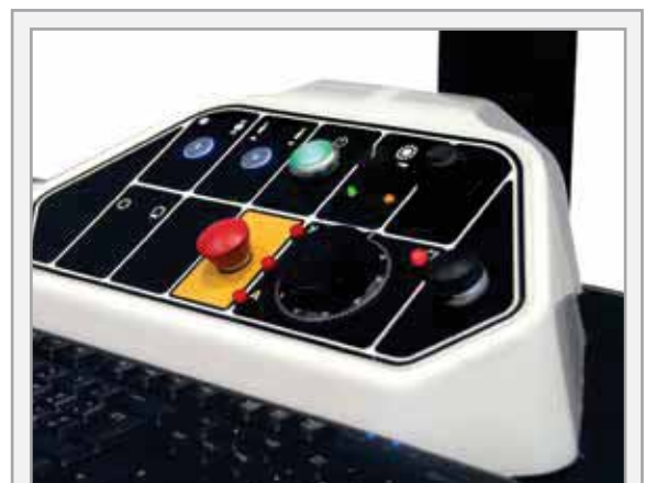
Micrometric hand-wheel, joystick and independent axes selection integrated in the control's cockpit for maximum ease of use and ergonomics.
