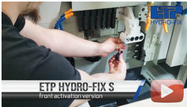
Front activation version in Drill arm application. Tool change in 30 seconds!
