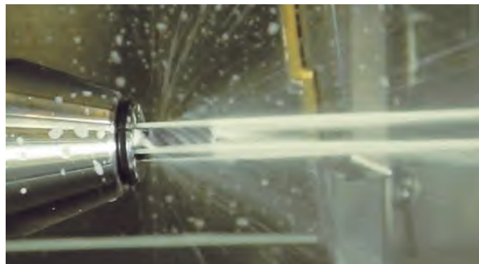
Using Reduction sleeve HS-CF - for peripheral cooling.
