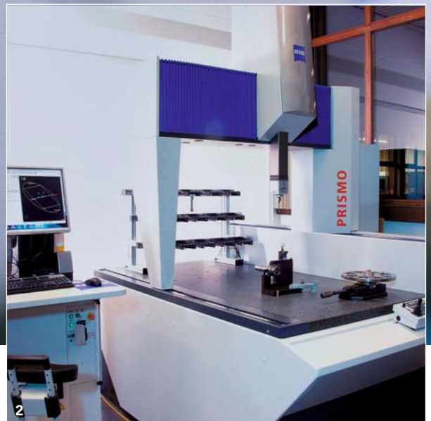
1: Roboteranlage/Robotic engineering 2: Messmaschine Zeiss/Measuring machine from Zeiss
