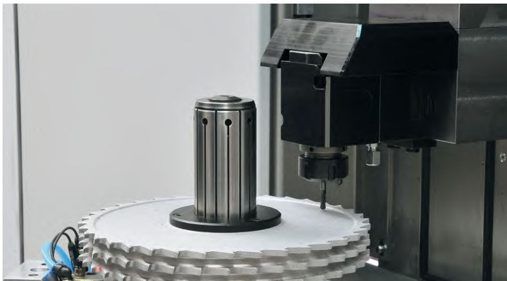
Balancing of PCD jointing cutters for laminate Balancing enables the best edge quality for the piece of furniture by vibration-free tool run. In addition, the noise while machining is reduced to a minimum.
