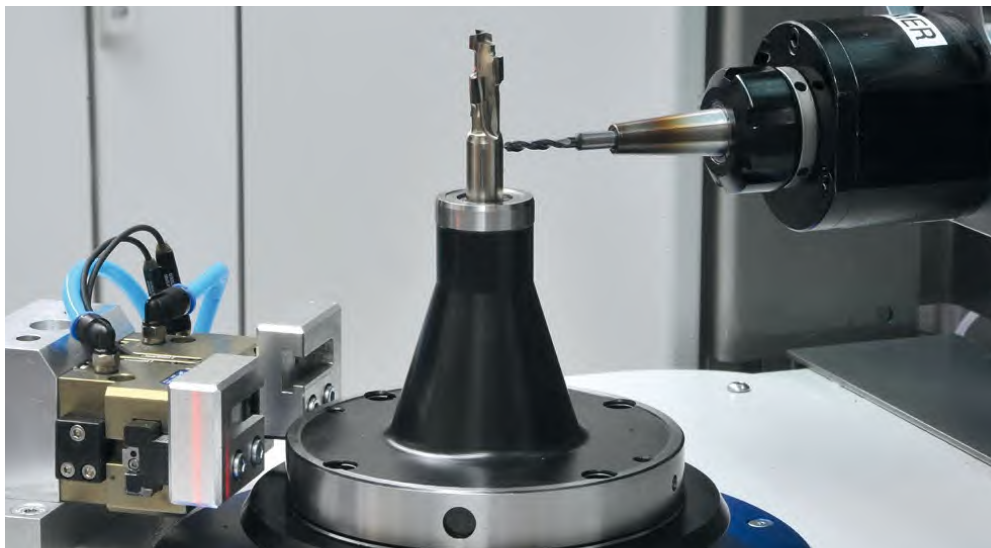
Balancing of tools with a HG balancing adapter for tools with a cylindrical shank For further information, please go to page 55.
