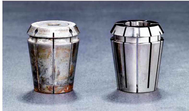
Two collets each after 4 months of use: The left one without coating – the right one with FAHRION|Protect
