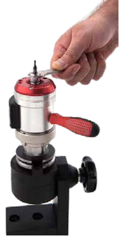
Figure 34: Loosening ER11 nut
