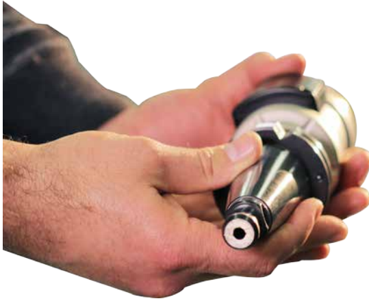
Figure 30: Example of a toolholder with a hole for coolant flow
