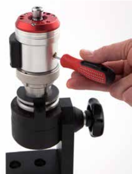
Figure 32: Inserting the WRENCH DIA3.2X45 into the HSM Jet Spindle
