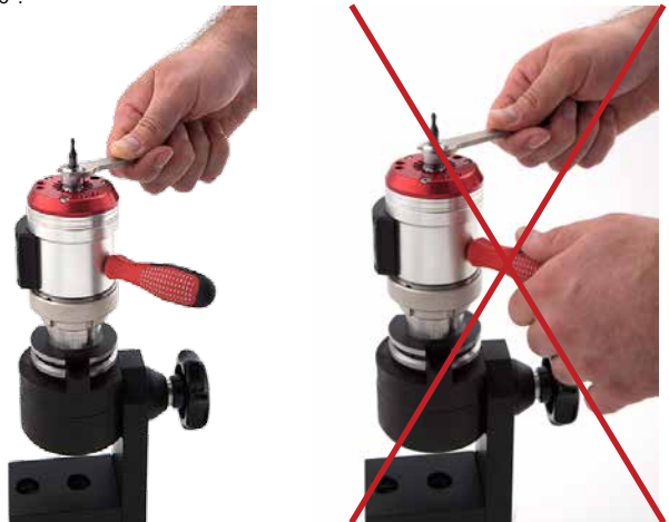
Figure 36: Tightening ER11 nut
