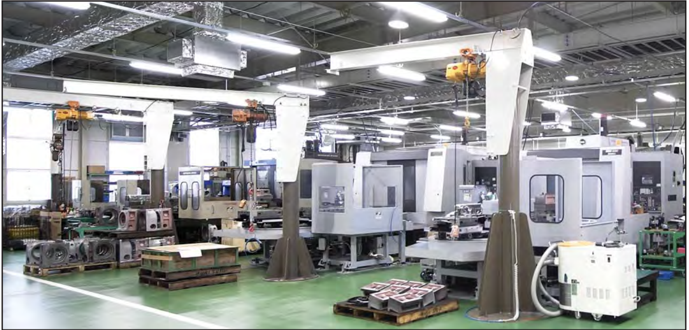
Machine Center Line with 3Lock Spindles
