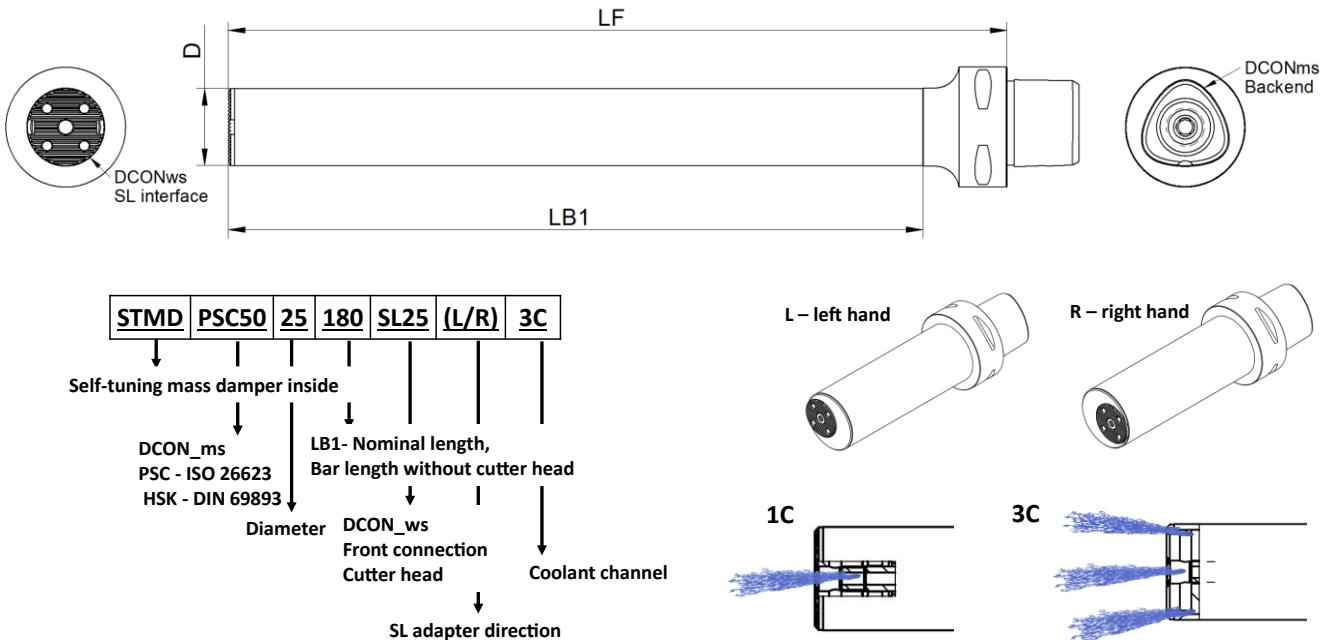
Standard: PSC32 (with SL interface and exchangeable heads)
