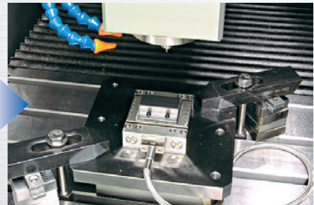
Measuring X/Y/Z cutting force by Dynamometer.
