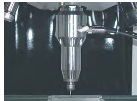
HES510 Spindle - Max. 50,000rpm
