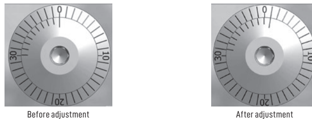
This Example Shows .001" Adjustment
