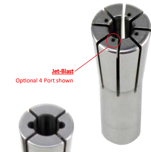
1/2 Moon Jet-Blast, only used when collet wall is too thin for full diameter Jet-Blast holes.
