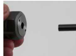
Insert cutting tool with the seal engaged on the round part of the shank
