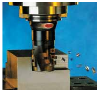
Power milling with Graflex® Modular System: metal removal rate 432 cm 3 /min
