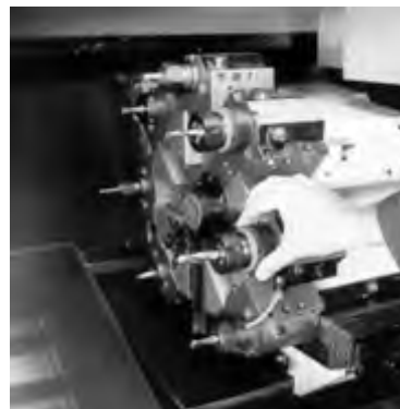
Rotate the Smith-Lock® Quick-Change nut in a counter-clockwise direction.
