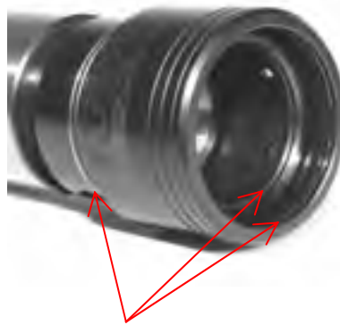
Contact seals to prevent corruption from entering the OSA & spindle bore.
