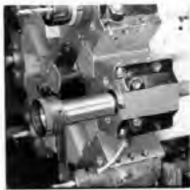
The Quick-Change Sleeve Adapter is inserted in the lathe tool holder and locked in place.
