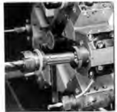
The Quick-Change Sleeve Adapter accepts T.M. Smith Tru-Taper® Drill Holders and Smith-Lock Conversion Adapter Nuts.
