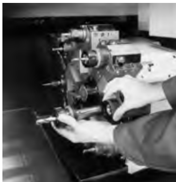
Insert the tool holder into the Adapter Sleeve.
