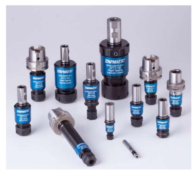
**SynchroFlex**® Tap holders for synchronized tapping cycles. For tap sizes M1 to M48. With high pressure, high volume internal coolant system. **SynchroFlex**® compensates for the unavoidable discrepancy between machine synchronization and actual tap pitch, dramatically improving tap life and thread quality.
