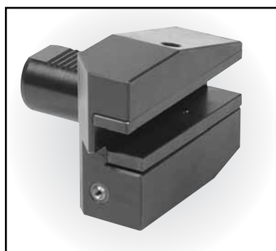
Toolholder with parallel shank and transversal rectangular seat, upside-down, left-hand long.
