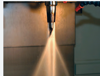
CoolBLAST coolant ports direct coolant on the tool path, even at high RPMs.
