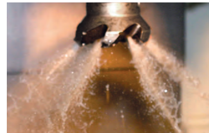
CoolBLAST arbor screw provides coolant path.
