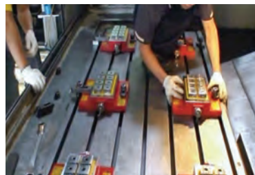
Position the chucks on the machine bed
