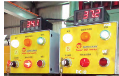
Controls require operator to use both hands
