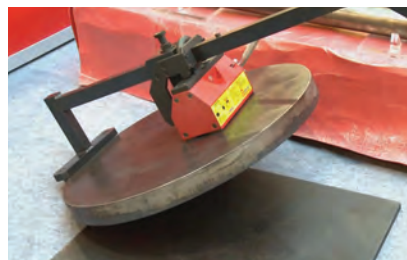
Move round or rectangular stock vertically
